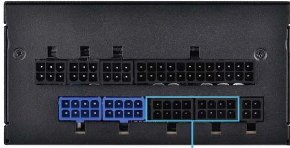
8 / 4-Pin EPS / ATX 12V connector x 2
