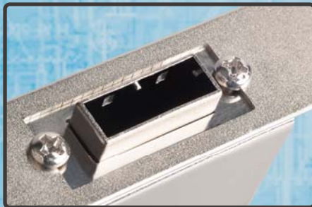
External : Mini-SAS SFF-8088 x 1 (to external drive enclosure, e.g. TS431S)
