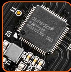
PCIe Gen2 x2 with ASMedia 1062R controller
